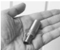
Fig.3: Through the use of modern micro electronic parts all functions are integrated in the sensor. No additional external amplifiers or switching boxes are necessary.
