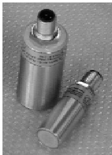
Fig.2: Singlesided sheet touching Double Sheet Sensors for steel sheets up to max. 0,5 mm thickness: Type S 0.5P4S diameter: 18 mm, length: 45 mm for steel sheets up to max. 1,0 mm thickness: Type S 1.0P3S diameter: 28 mm, length: 55 mm for aluminium sheets up to max. 0,5 mm thickness: Type SA 0.5P3S diameter: 28 mm, length: 55 mm
